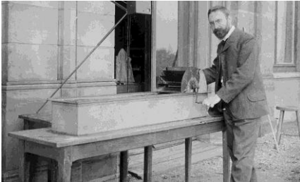
Ludwig Prandtl 1904 - 1,5m water test channel Picture: Estate administration University of Göttingen (Germany)
